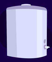
A hot water cylinder is a well-insulated tank which stores water after it's been heated. Water is heated through your heat pump system and is then stored, at a temperature, ready for you to use whenever it's needed. This is typically found on the ground or first floor of your home (the closer to the outside the better). But yours may be installed in a different spot such as the loft.
